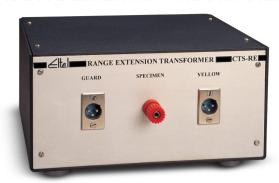
The Range Extension Transformer Model CTS-RE is an accessory for ACTS-12K & ACTS-12K PLUS Capacitance & Tan Delta Test Sets. The CTS-RE extends the Capacitance measuring range of the ACTS-12K & ACTS-12K PLUS by a factor of ten (10), from 0.26mF to 2.6mF.
