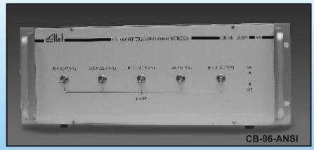
**Description**: The ANSI Current Transformer Burden Model CB-96-ANSI is designed for loading the Current Transformers during accuracy tests .The ANSI Burden is designed as per ANSI Standard C57.13. It can be used alongwith the Eltel Automatic Instrument Transformer Test Set AITTS-98 to test CTs as per ANSI Standards. The AITTS-98 Test Set directly displays the Ratio Correction Factor(RCF) while testing CTs.
